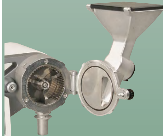
Milling chamber with Safety switch, funnel, lid, rotary slide for product dosage and NS29 adapter for intercepting tubes
