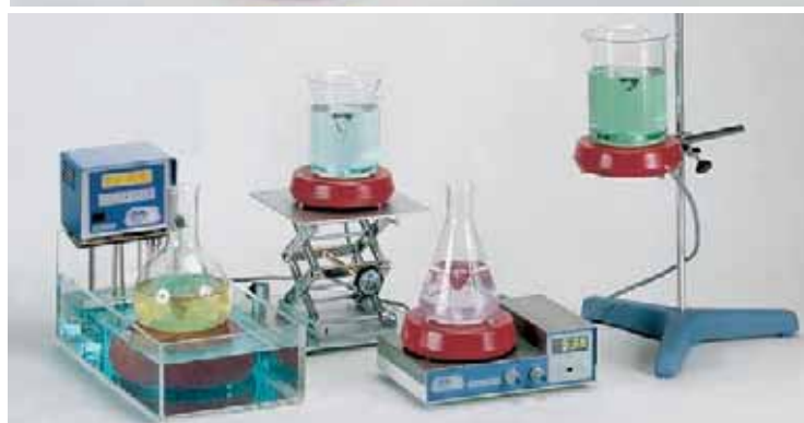
Example: system of submerged stirrers table top and with retort stand.
