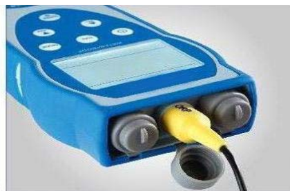
Sealed Connector for Waterproof
